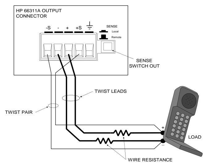
2. Is the resistance of the load leads, sense leads, and any external relays less than 2 ohms per lead (or per side) between the dc source and the phone contacts? Check the resistance of the lead path.
